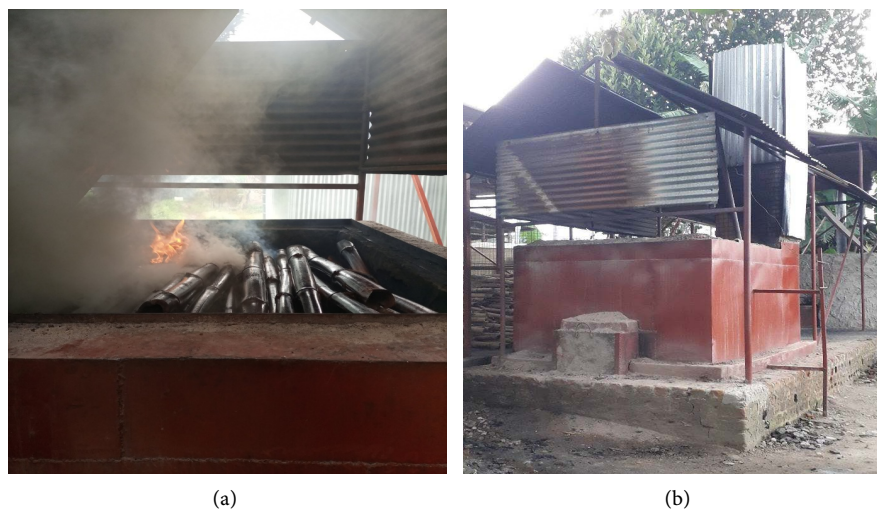
Figure 1. (a) Bamboo carbonization; (b) Carbonizer left to cool.
