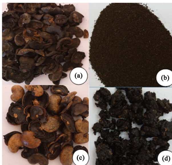
Figure 2. Photograph showing condition of two types of sample of cashew hulls: (a) Old hulls; (b) Powdered old hulls; (c) Fresh hulls; (d) Crushed fresh hulls.
