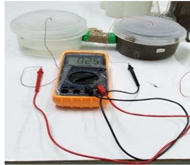
**Figure 1.** Double chamber microbial fuel cell setup [13].
