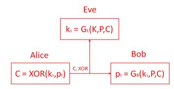
**Figure A1.** Information flow.  $G_B$ : Bob's Grover searching algorithm following **Appendix 1**, substituting XOR [33] for the encryption algorithm E in Equation (10).  $G_E$ : Eve's Grover searching algorithm following Section 5.11, substituting XOR [33] for the encryption algorithm E in Equation (6).
