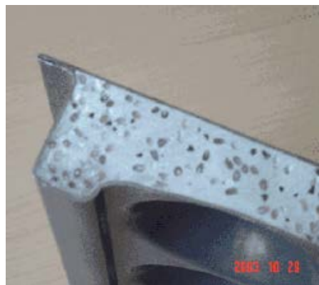
Figure 7. Filling of phase-change material.
