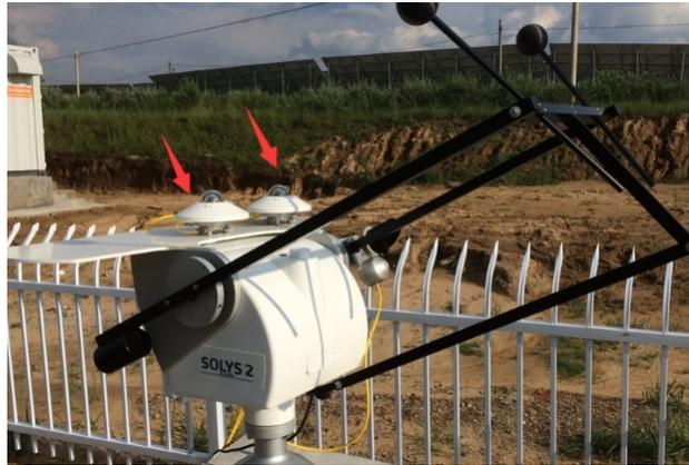
**Figure 3.** Solar tracker and direct radiometer.
