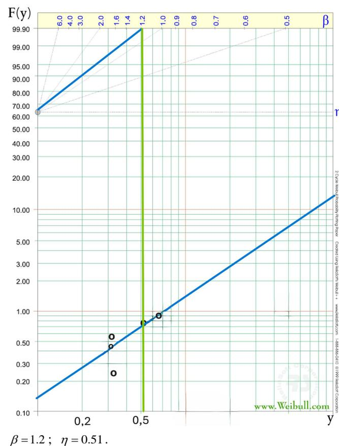
**Figure 4.** Example of Grafical models of Weibull data distribution for indications of the object “Welded joint on the outer surface of the reactor vessel of the power unit” 1997.
