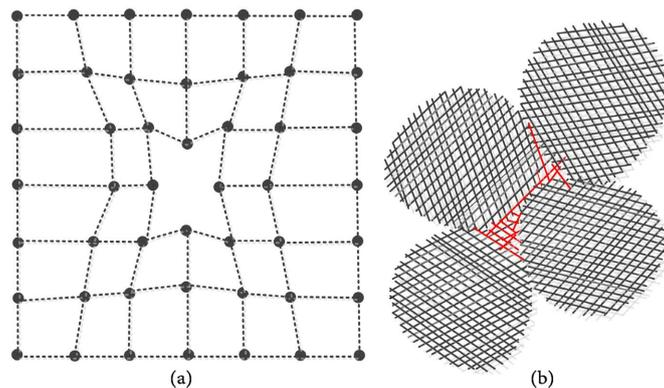
**Figure 1.** (a) Scheme of vacancy in the crystal metal lattice. (b) Scheme of a mosaic structure in real metal.
