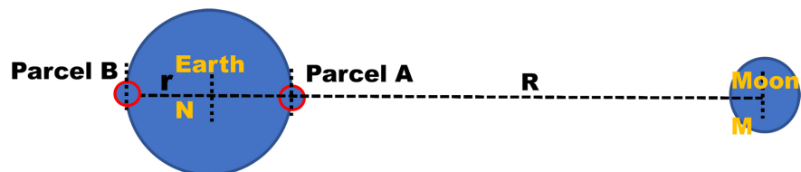
Figure 1. There are four objects in a universal system. The distance between the Earth's centroid and the lunar centroid is R , and the distance between the oceanic fluid parcel A (parcel B) and the Earth's centroid is (Earth's radius) r .
