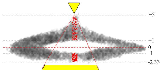
**Figure 3.** The  $\theta$ -based model of spin deflection in the Stern-Gerlach experiment is driven with random spin vectors and trajectories are calculated. The red dots representing individual particles are overlaid on the gray SG data from the iconic postcard. The scale has been chosen to facilitate the overlay. The Stern-Gerlach magnets are diagrammed in yellow. Horizontal spreading of the red data points is for illustrative clarification and is not physically meaningful.
