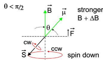
**Figure 4.** Spin  $s$  and magnetic moment  $\mu$  in inhomogeneous magnetic field  $B$  with spin down.
