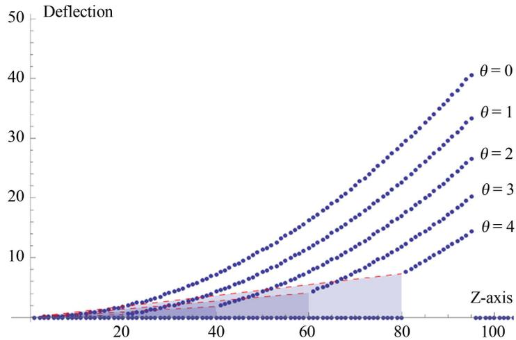
**Figure 2.** The  $\theta$ -dependence for small angles is shown. Shaded areas below the dashed red lines represent the alignment process during which the initial spin enters the field with angle  $\theta$  and proceeds to align with the local field. After alignment the gradient force accelerates all particles equally, seen as dotted blue lines. Scales have been chosen to enhance the different deflections. Actual scales depend upon field strength, field gradient, length of travel, and geometry.
