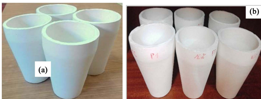
Figure 1. Pictures (a) green crucibles and (b) sintered crucibles.
