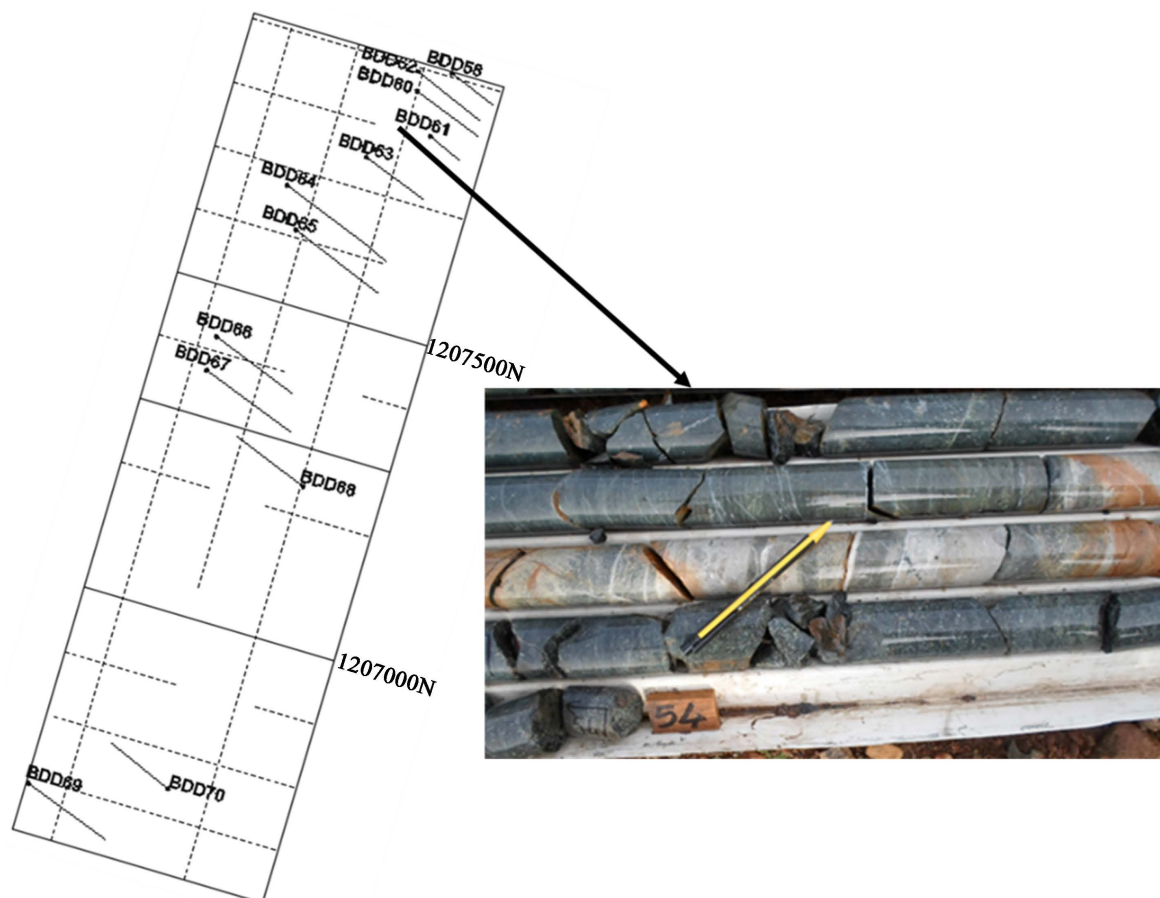
Figure 2. Location of core drilling collars in the IntiéDougou target with a photograph of a core box.
