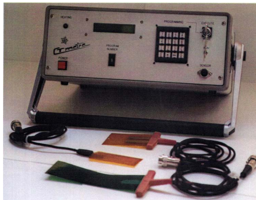
Figure 6. Device for thermal conductivity test.
