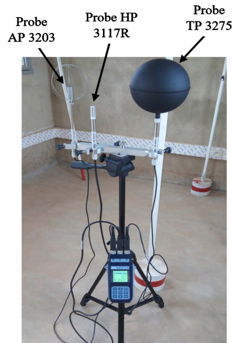
Figure 2. Delta OHM type HD32.3 hydrothermal measuring equipment.
