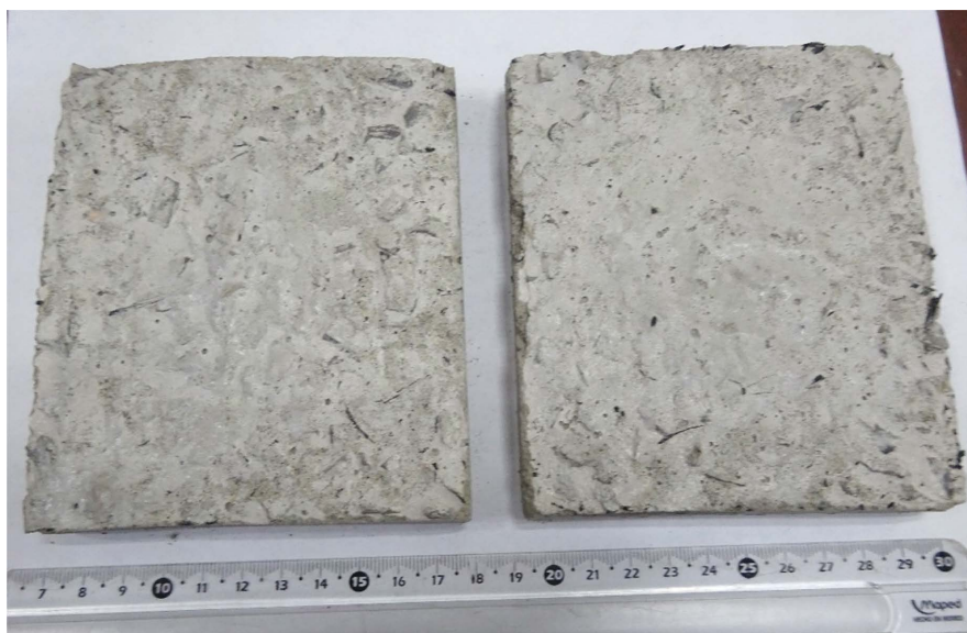
Figure 2. Example of the platelets obtained after 24 h of setting.
