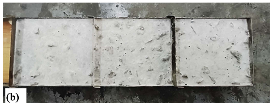
Figure 1. (a) Wooden base mold and steel spacers. (b) Samples cast in the mold.
