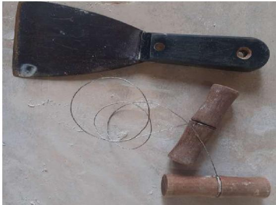
**Figure 6.** Scraper and cutting wire.
