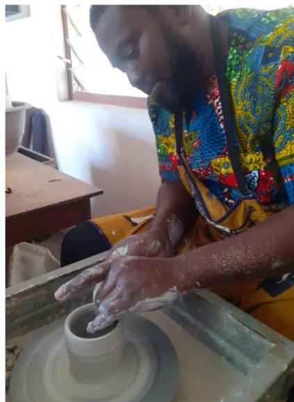
**Figure 22.** Pulling of centred ceramic body (Source: Field work, 2023).
