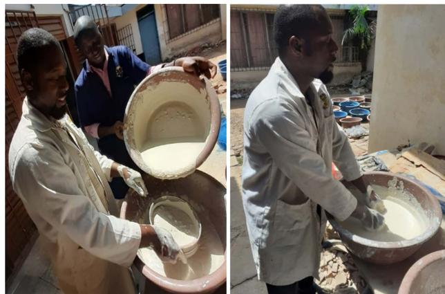
**Figure 14.** Series of sieving of mixture to obtain creamy body (Source: Field work, 2023).
