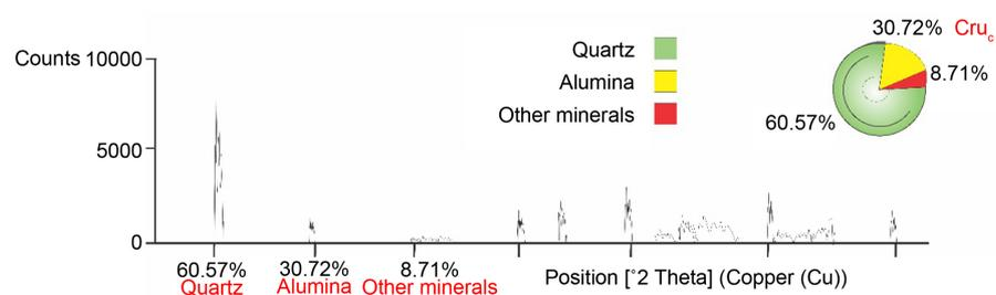
**Figure 19.** Results of XRF pattern for composition Cru<sub>c</sub>. (Source: Field work: GSA: 2023).
