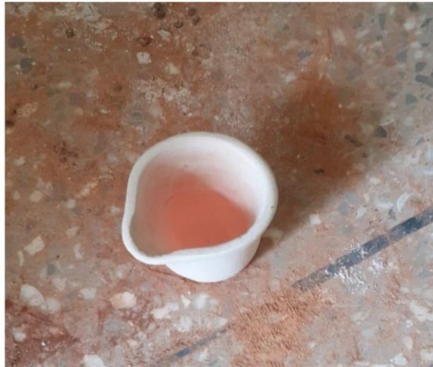
**Figure 27.** Hot crucible after passing the thermal shock test.
