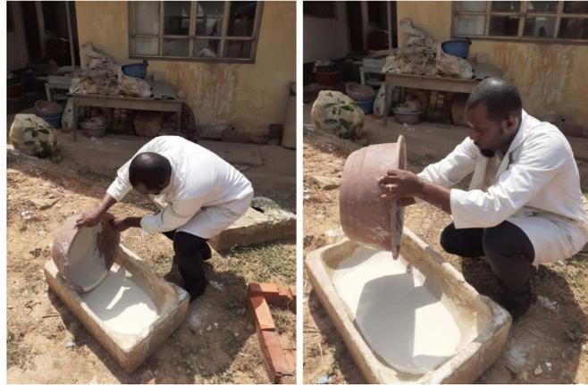
**Figure 15.** Pouring of creamy body into moulds (Source: Field work, 2023).
