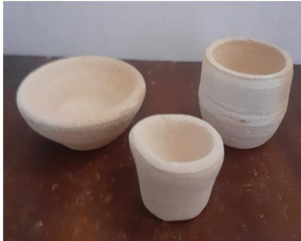
**Figure 24.** Crucibles sintered at 1400°C.
