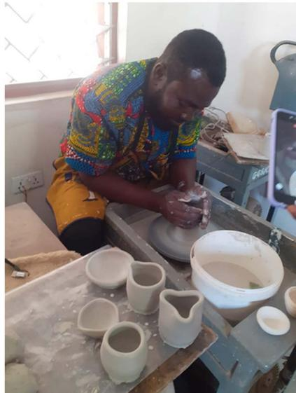
**Figure 21.** Centering of ceramic body (Source: Field work, 2023).
