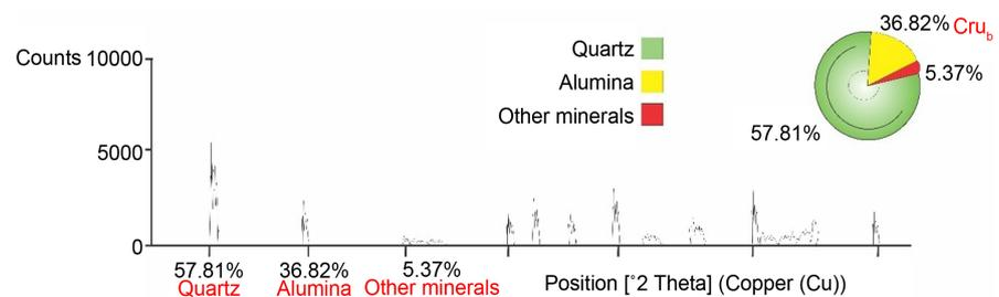
**Figure 18.** Results of XRF pattern for composition Cru<sub>b</sub> (Source: Field work: GSA: 2023).
