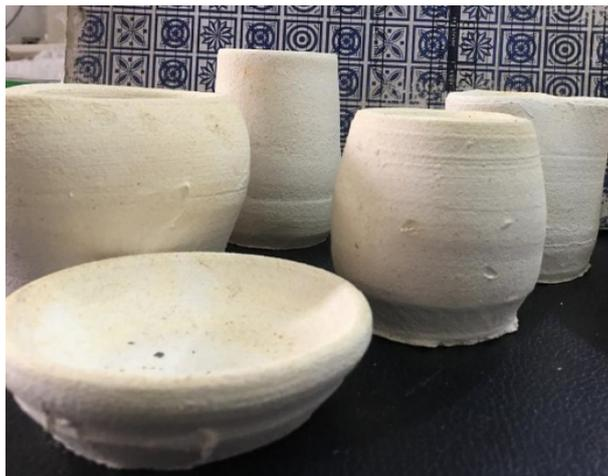
**Figure 25.** Crucibles sintered at 1500°C.
