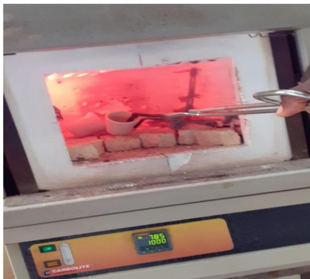
**Figure 26.** Testing for thermal shock in the crucible.
