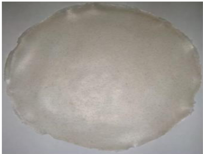
Figure 6. Biocomposite based on maize starch reinforced with kenaf fibers [8].
