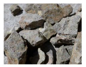
**Figure 4.** Cryptocrystalline structure basalt from Suluu-Terek deposit (image resolution  $8 \times 8$  cm).
