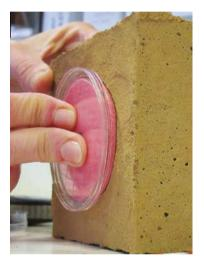
Figure 9. Sponge contact test principle [14].
