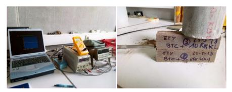
Figure 7. Measurement of thermal conductivity of CSEB after 14 and 28-days cure.
