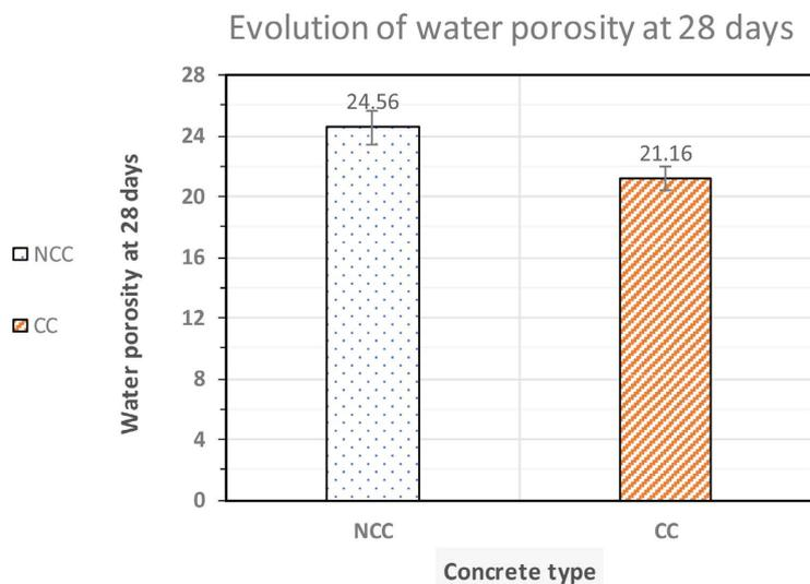
Figure 6. Evolution of porosity before and after carbonation.
