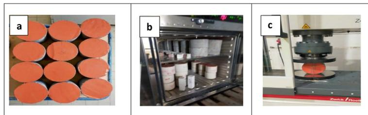
**Figure 2.** Shows: a) preparation of specimens filmed on both cross-sectional faces to impose CO<sub>2</sub> diffusion in one direction only; b) placing of specimens in the carbonation chamber; c) breaking of specimens by splitting to spray phenolphthalein.
