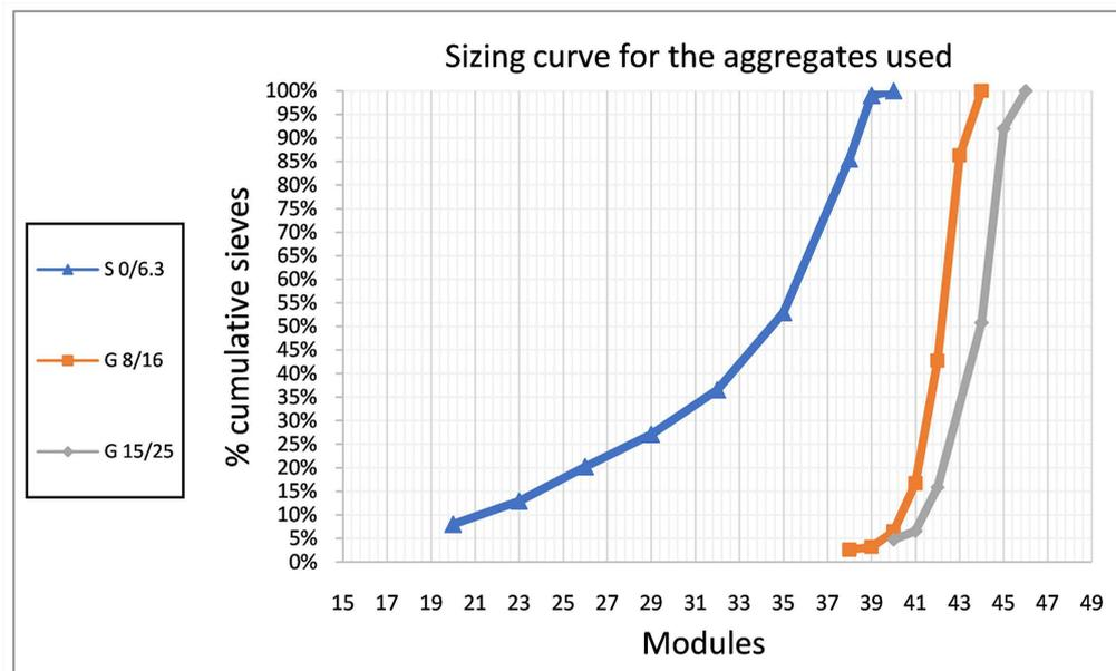
**Figure 1.** Sizing curve for the aggregates used.
