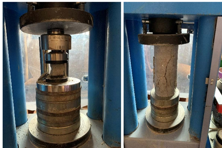
Figure 3. Compression tests on Mortar and concrete specimens.
