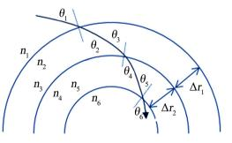
Figure 2. Light refraction by gravitational field.
