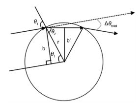
Figure 3. A slightly refracted light path at the boundary of different matter.
