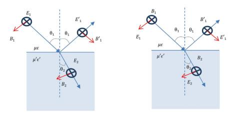
Figure 4. left: s-polarization (TE mode), right: p-polarization (TM mode).
