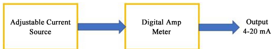
Figure 2. Block diagram of the 4-20 mA calibrator.
