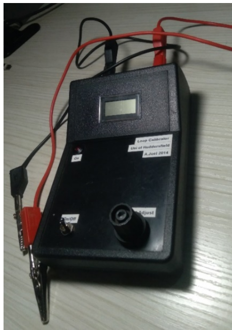
Figure 13. The 4-20 mA loop calibrator prototype.
