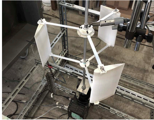
Figure 9. Photograph of the VAWT test model in the test section downstream of the wind tunnel.
