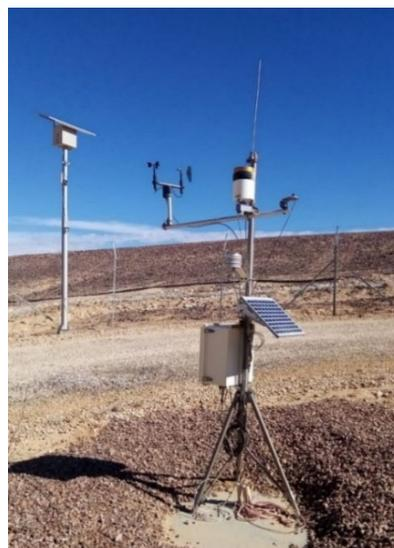
**Figure 3.** Weather station inside the power plant.
