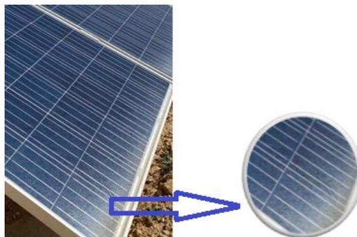
**Figure 5.** Accumulated dust on a PV surface.
