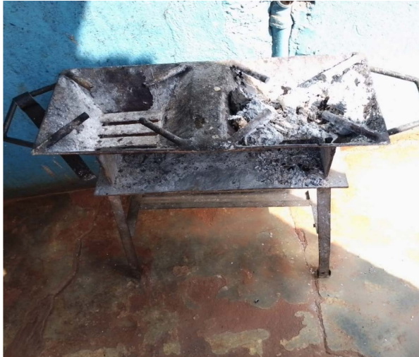
Figure 3. Two-plate scrap metal charcoal stove. (Source: Author).
