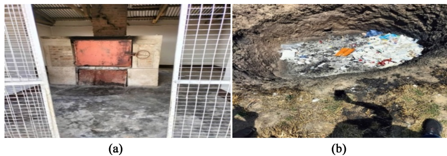
Figure 6. Different Burning Structures in Healthcare Facilities. (a) Burning Structure in one HCF in Sumbawanga Town Council; (b) Open Air Burning in one HCF at Nkansi DC.
