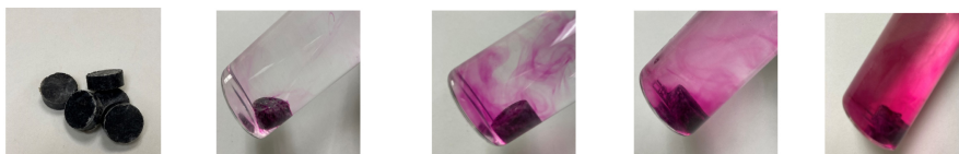
Figure 2. CRBP pellet with \text{KMnO}_4 encapsulated inside PCL and its diffusion in reagent grade water over time.
