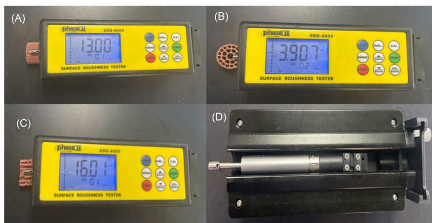
Figure 7. (A): R_a value of the outermost features; (B): R_a value of the lateral view section; (C): R_a value of the cross-section; (D): Bottom view of the SRG-4000 surface roughness tester.
