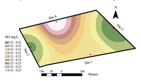
Figure 4. Oxygen dissolved distribution according to ArcGIS software in the leachate lagoon.
