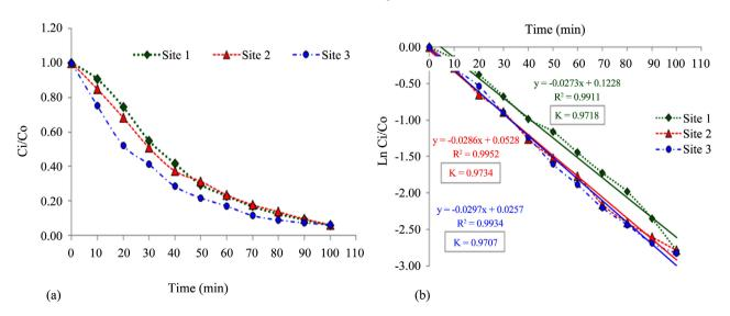
Figure 6. (a) Kinetics curves profile resulting from ozone-UV oxidation. (b) First order kinetic runs.
