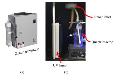
Figure 2. (a) Ozone generator. (b) Ozone-UV combined system.
