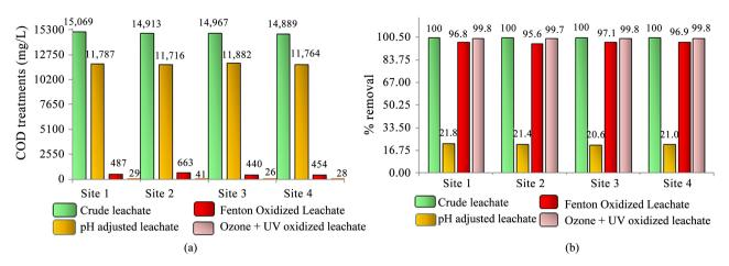
Figure 7. (a) Treatments stages. (b) COD removal efficiency in each treatment.
