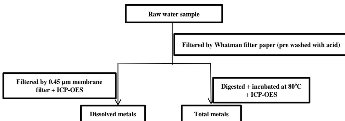
Figure 2. Metal speciation scheme for water samples (Schwarz, 1977).
