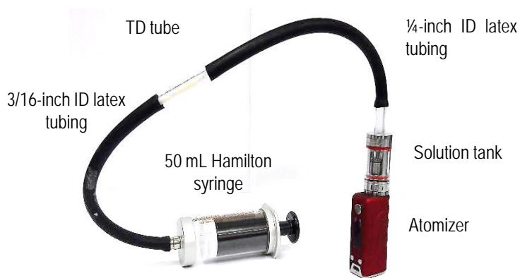
Figure 1. Apparatus set-up for aerosol sampling consists of 50 mL Hamilton air-tight syringe, latex tubings, TD tube and e-cigarette devices [5].
