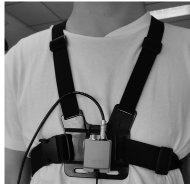
Figure 2. Inertial sensor wear schematic.
