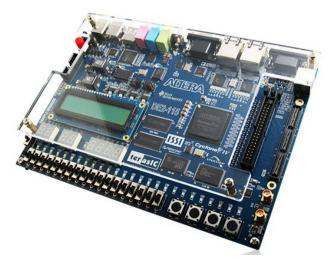
Figure 4. Altera cyclone IV 4CE115 FPGA device [13].
