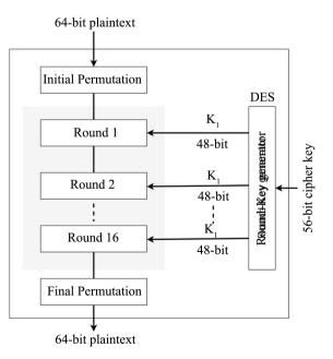
Figure 1. Overview of DES algorithm [6].
