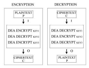
Figure 2. Overview of 3DES algorithm [7].
