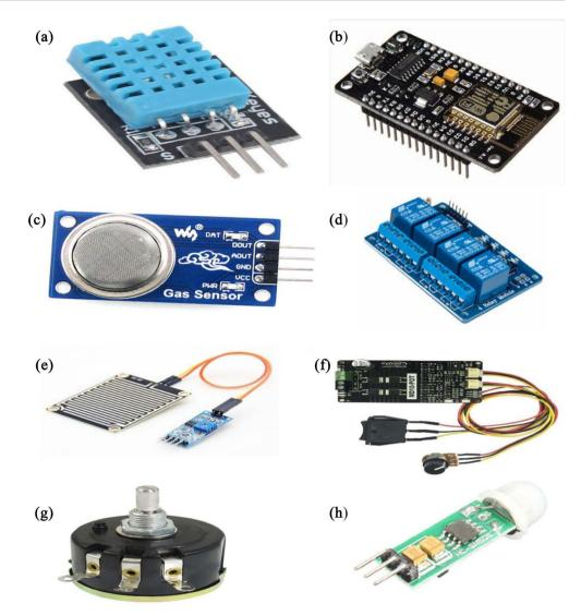
**Figure 4.** Components used in this experiment. (a) DHT11; (b) Node-MCU; (c) MQ2; (d) 4-channel relay module; (e) Rain sensor; (f) MD-10 POT; (g) Potentiometer; (h) PIR motion sensor.
