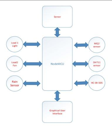
Figure 2. Schematic diagram of the proposed architecture.
