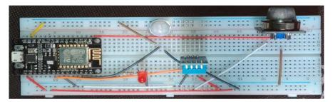
Figure 6. Breadboard assembly of smart home prototype.
