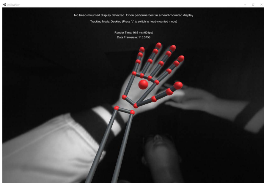
Figure 6. Missing information capture by Leap Motion due to finger occlusion.
