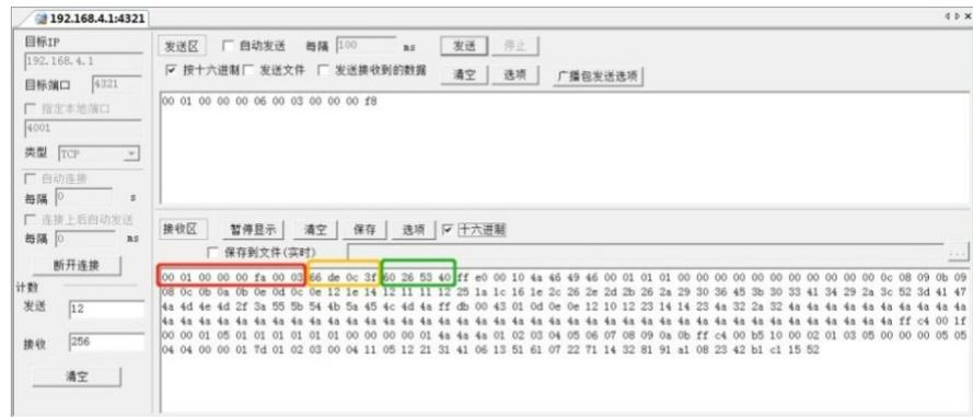
**Figure 7.** MODBUS-TCP sending query response process.
