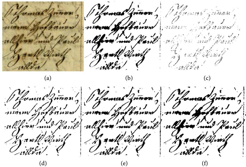
**Figure 7.** (a) Inputted image (DIBCO 2016); (b) Result of Otsu technique; (c) Result of Sauvola's technique; (d) Result of Nick's technique; (e) Result of local adaptive thresholding; (f) Result of proposed technique.
