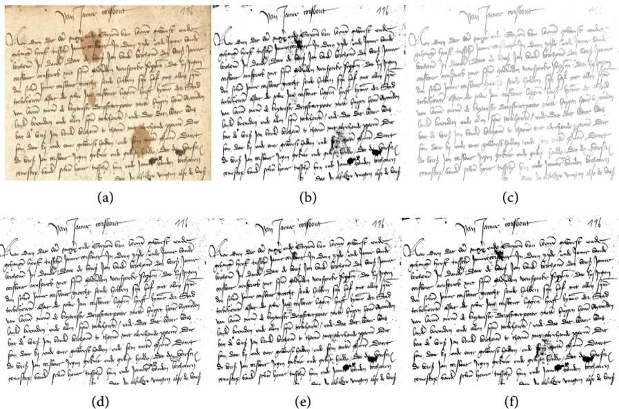
**Figure 8.** (a) Inputted image (DIBCO 2017); (b) Result of Otsu technique; (c) Result of Sauvola’s technique; (d) Result of Nick’s technique; (e) Result of local adaptive thresholding; (f) Result of proposed technique.
