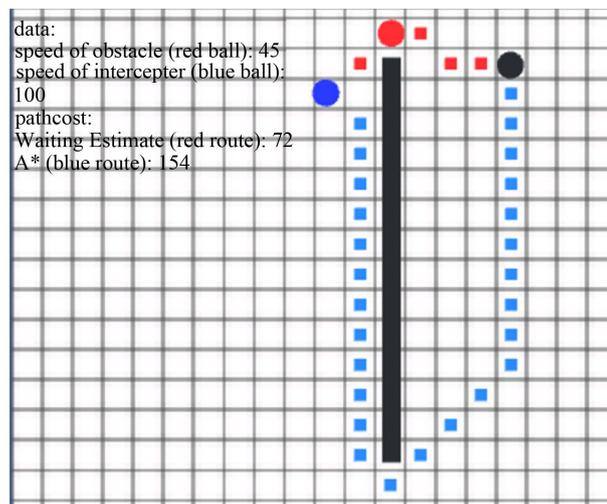
**Figure 7.** Comparison of the two algorithm paths.
