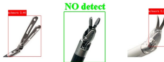
Figure 2. Object detection using pre-trained dataset and YOLO-local-application.
