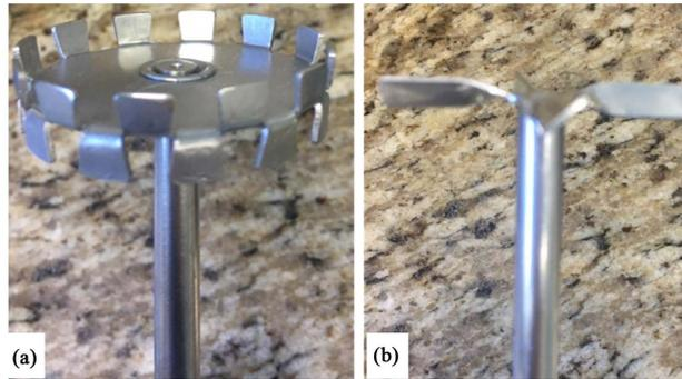
**Figure 1.** Rods used to optimize the preparation of nanoemulsions: (a) cog (H1) and (b) helix (H2).
