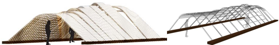
Figure 21. A perspective illustrates the different configurations of the space depending on the degree of bending of the wooden tapes according to the degree of humidity (Second Movement).
