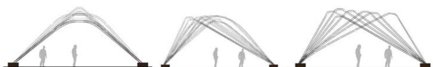
Figure 15. Vertical-side projections of the three movements proposed for the Pavilion design according to the humidity change degree.
