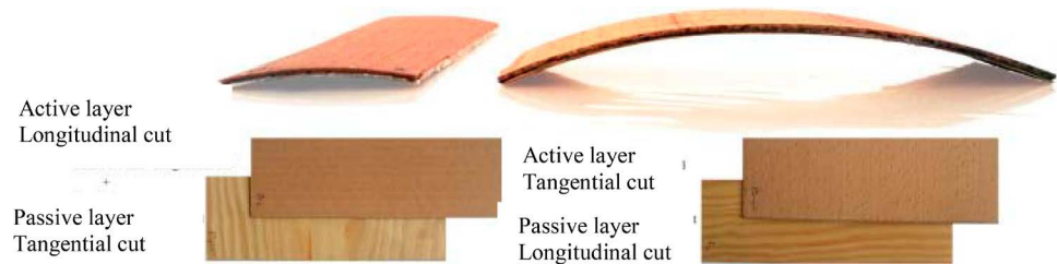
Figure 3. Hygroscopic behavior of thin Pine Veneer material.
