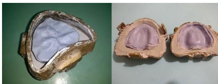
Figure 3. The silicone mold in the flask, first the lower half (left) and then the upper one. On the right, the opened hybrid flask.
