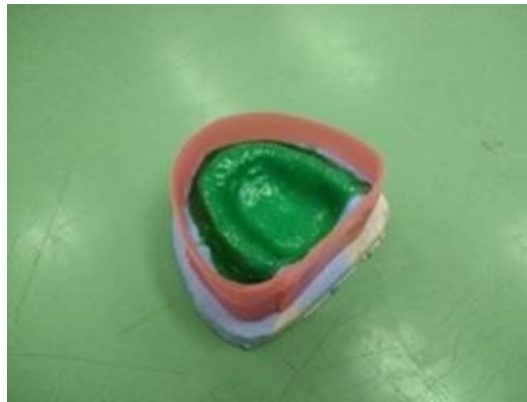
Figure 1. Illustration of the boxed cast in order to fill in with silicone.
