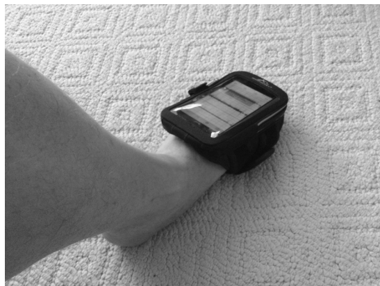
Figure 1. Illustration of the mounting procedure for the smartphone representing a wearable and wireless gyroscope platform about the dorsum of the foot and supported by an armband.
