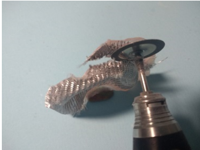
Figure 5. The cutting of the excess mesh using a thin metal disk.
