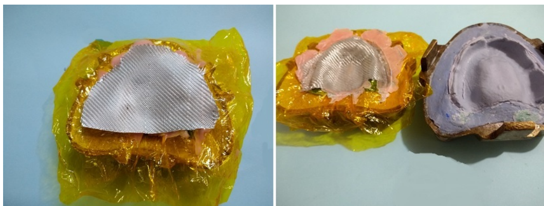
Figure 3. Contouring of the fiber mesh with self-polymerizing resin under pressure in the modified mold.
