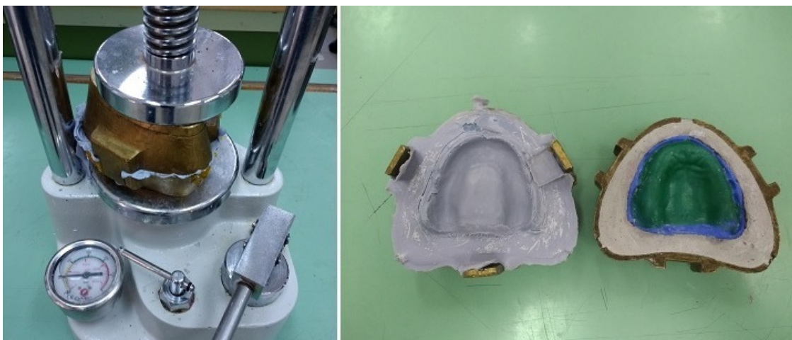
Figure 2. Modification of the upper half of the mold with silicone impression putty.
