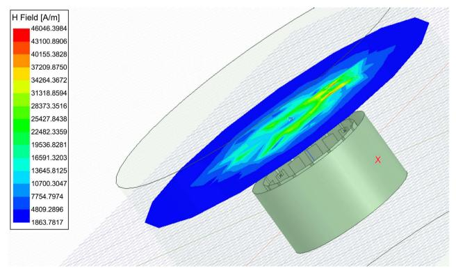
Figure 6. A different setting of a Birdcage coil simulation that may be accommodated for wearable devices. Notice H-field is a little above the birdcage coil.
