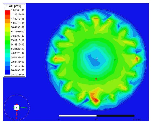
Figure 7. The E-Field distribution over the head phantom.
