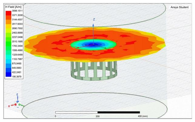
Figure 3. Displaced conductors more than 10 mm will cause H-field and accordingly EM energy to escape from the Birdcage system.
