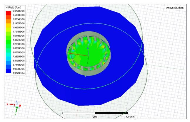
Figure 4. The H-field distribution inside the Birdcage coil.
