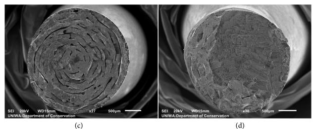
**Figure 3.** SEM images of selected representative fractured specimens post-welding: (a) Ni-Cr with Argon, (b) Ni-Cr without Argon, (c) Co-Cr with Argon, (d) Co-Cr without Argon.
