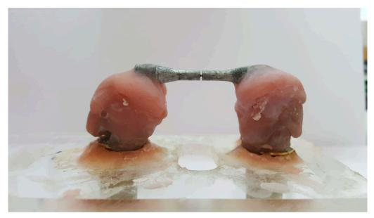
**Figure 2.** The cut area and the formation of the cones are displayed. The corresponding laser welding wire was used to fill the gaps created.
