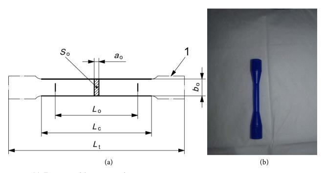
**Figure 1.** (a) Illustration of the specimen, from <u>https://regbar.com/wp-content/uploads/2019/09/ISO-6892-1-2009.pdf</u> (b) Wax specimen manufactured via CAD/CAM (subtractive manufacturing).
