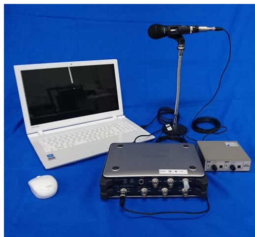
Figure 3. Fast Fourier transform analyzer and direction microphone.
