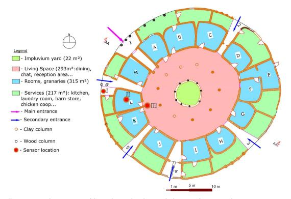
Figure 5. Spatial organization of the impluvium hut showing the location of measuring devices.
