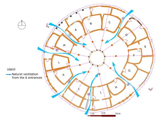
**Figure 8.** Horizontal section of the impluvium hut showing natural ventilation system. The rooms are indiquated by alphabetic letters allowing to locate the room (L).
