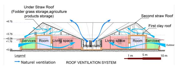
Figure 9. Vertical section of the impluvium hut showing the role of the main roof in the natural ventilation system.
