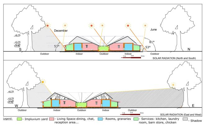
Figure 12. Study of sunshine on the impluvium hut.
