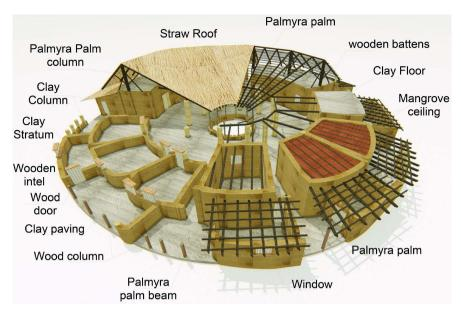
Figure 6. Constructive device and materials.
