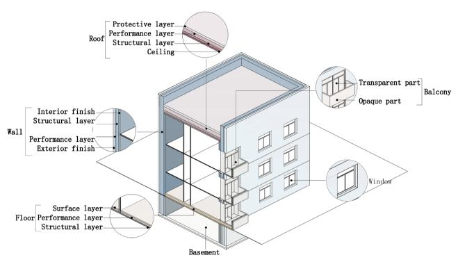
Figure 2. The parts and layers of the existing residential envelope system.
