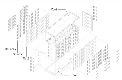
Figure 5. Layer of building-21 envelope system.
