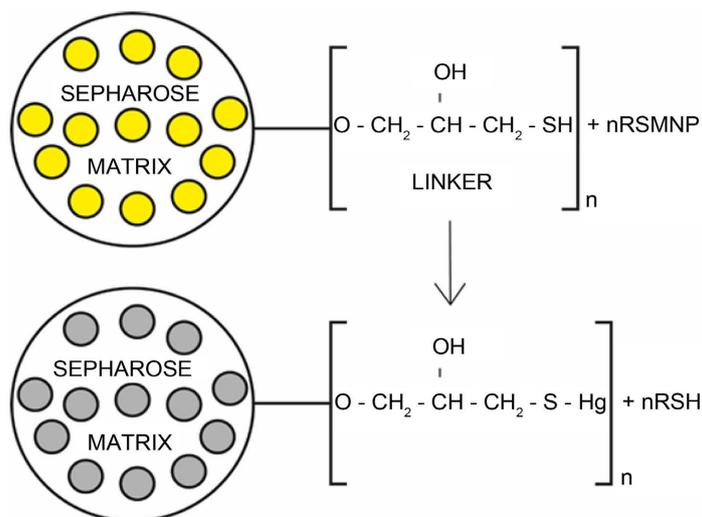
**Figure 2.** Use of an immobilized thiol column (TPS) to release a thiol from its mercurial adduct.
