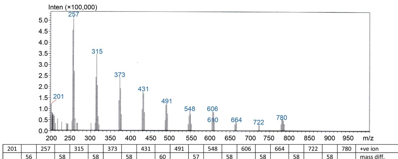
**Figure 7.** MS positive ions for peak eluting at 0.4 mins showing mercuri clusters and mass differences in stepwise fragments released.
