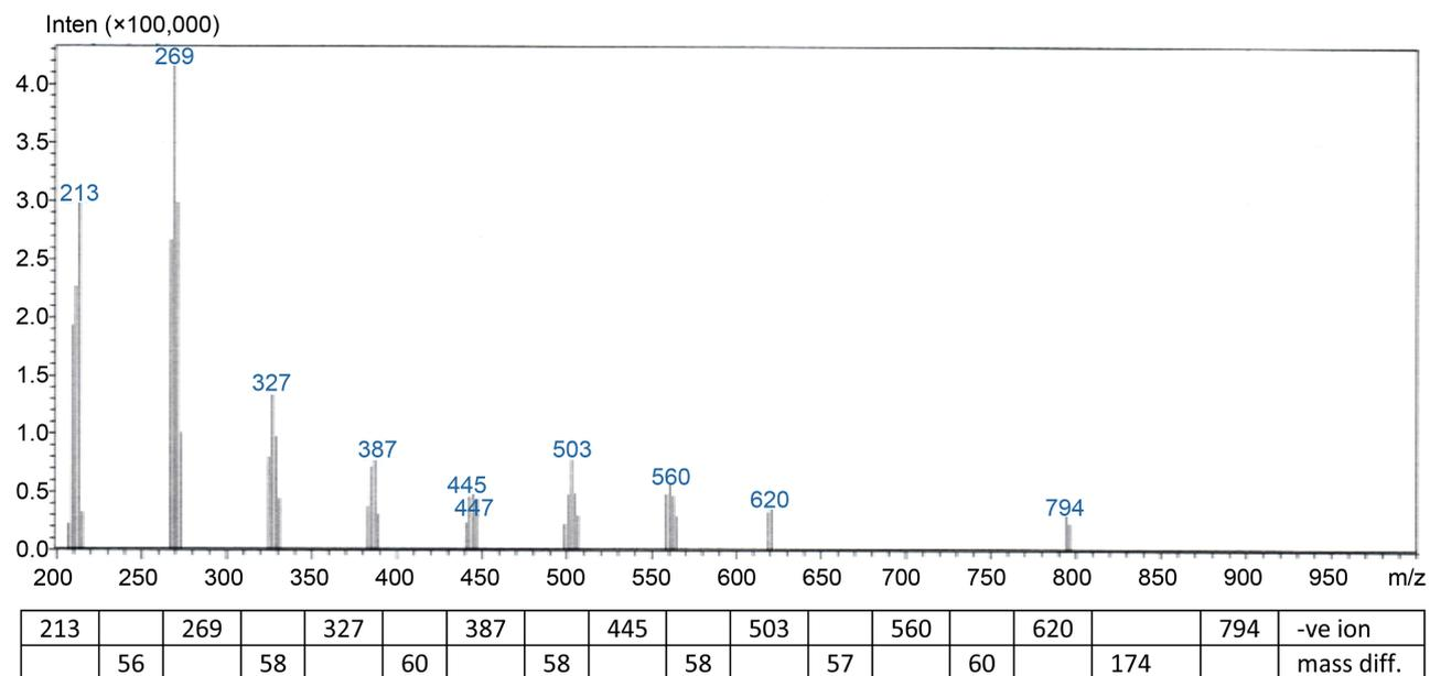
**Figure 8.** MS negative ions for peak at 0.4 mins showing mercuri clusters and mass differences in stepwise fragments released.
